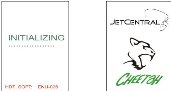
When the POWERPACK / ECU is connected to the HDT, the ECU battery is connected and the RX power is turned on, the HDT display screen will briefly display "INITIALING" with the software version of the HDT displayed across the bottom of the display, and then briefly displays the Logo of the turbine that is connected, after a few seconds the main screen will be displayed.
