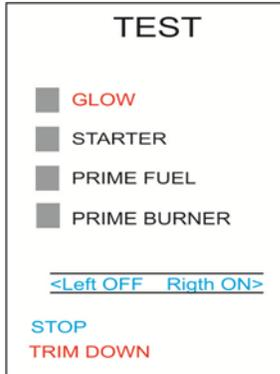
This screen features diagnostic tools to aid in the installation and testing the various turbine systems, in particular the priming of the fuel and burner lines.
