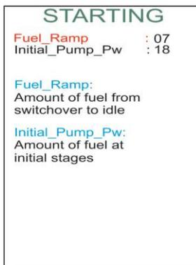
There are only two adjustable parameters in this sub-menu, “Fuel Ramp” values and “Initial Pump Pw”.
